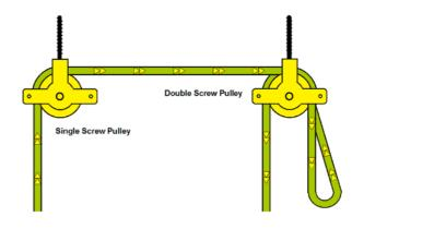
8 Raise each rack end so that it is flush with the ceiling and tie a knot in the loop of the rope at chest height. Lower the airer tying further knots at 40cm intervals until all the rope is tided away.
